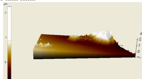
Figure 8a: 3D-image of surface morphology of \text{TiO}_2 thin film after the evaporation process using AFM.
